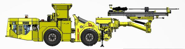
Width : 1.15 m Height : 1.90 m Weight (Operationnal) : 6,4 t ( a vérifier Parts, Operation and maintenance in PDF and USB key
