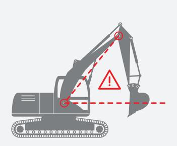
On/Off solenoid valves, proportional valves, and electrical motion control are all supported. Valves are not supplied. Where proportional valves are used, there are adjustable slow-down angles and equipment speed settings to provide a controlled soft-stop to the equipment. SS1 also has the added benefit of an internal warning so the operator is always aware of the limit. Angle measurement is courtesy of a gyro compensated solid state sensor with near direct drive performance.
