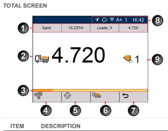
1 Data list display 2 Short Total 3 Weighing progress bar 4 Main Menu 6 Target weighing 6 Split weighing 7 Undo 8 Notification bar 9 Bucketloads
